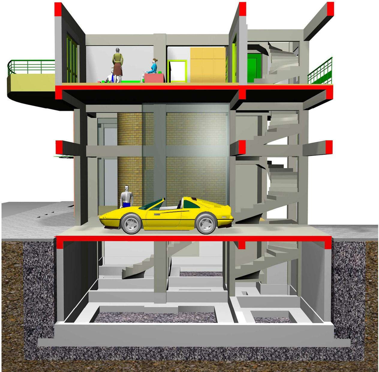
*In every building like the one shown in the above figure, permanent (dead) and imposed (live) loads are applied. The latter are much lower than the former, for example 3 persons and the living-room furniture weight as much as a single m<sup>2</sup> of slab surface while a car weights as much as a sole beam.*
