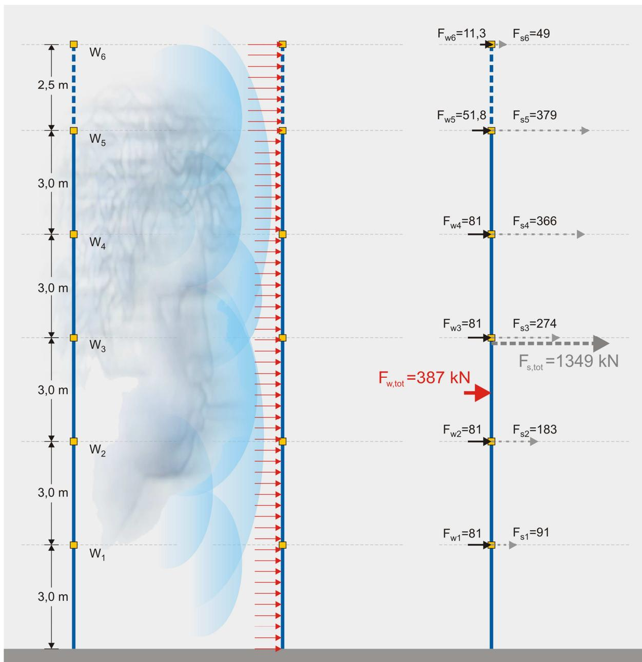
Figure 2.5-2: Wind forces  $F_w$  are less significant comparing to earthquake forces  $F_s$ .
