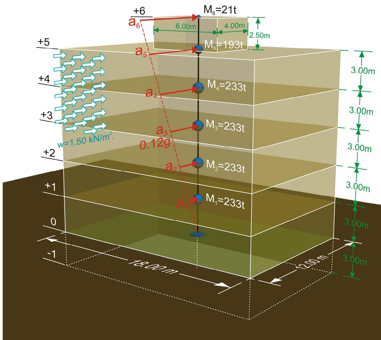
Figure 2.5-1: The geometrical and loading model of the building's wind and earthquake actions
