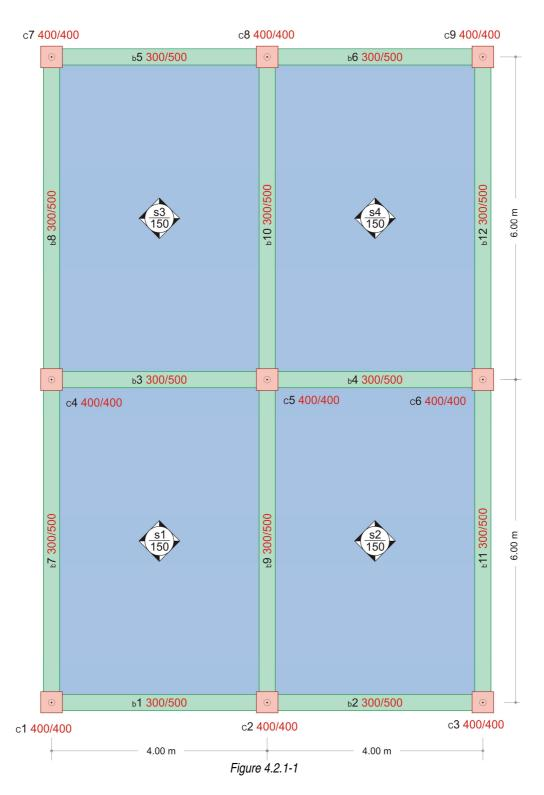
The four slabs have identical dimensions of 4.0 mx6.0 m, thickness of 150 mm, covering load  $g_e=1.0 \text{ kN/m}^2$  and live load q=5.0 kN/m<sup>2</sup>. Concrete class: C30/37.
