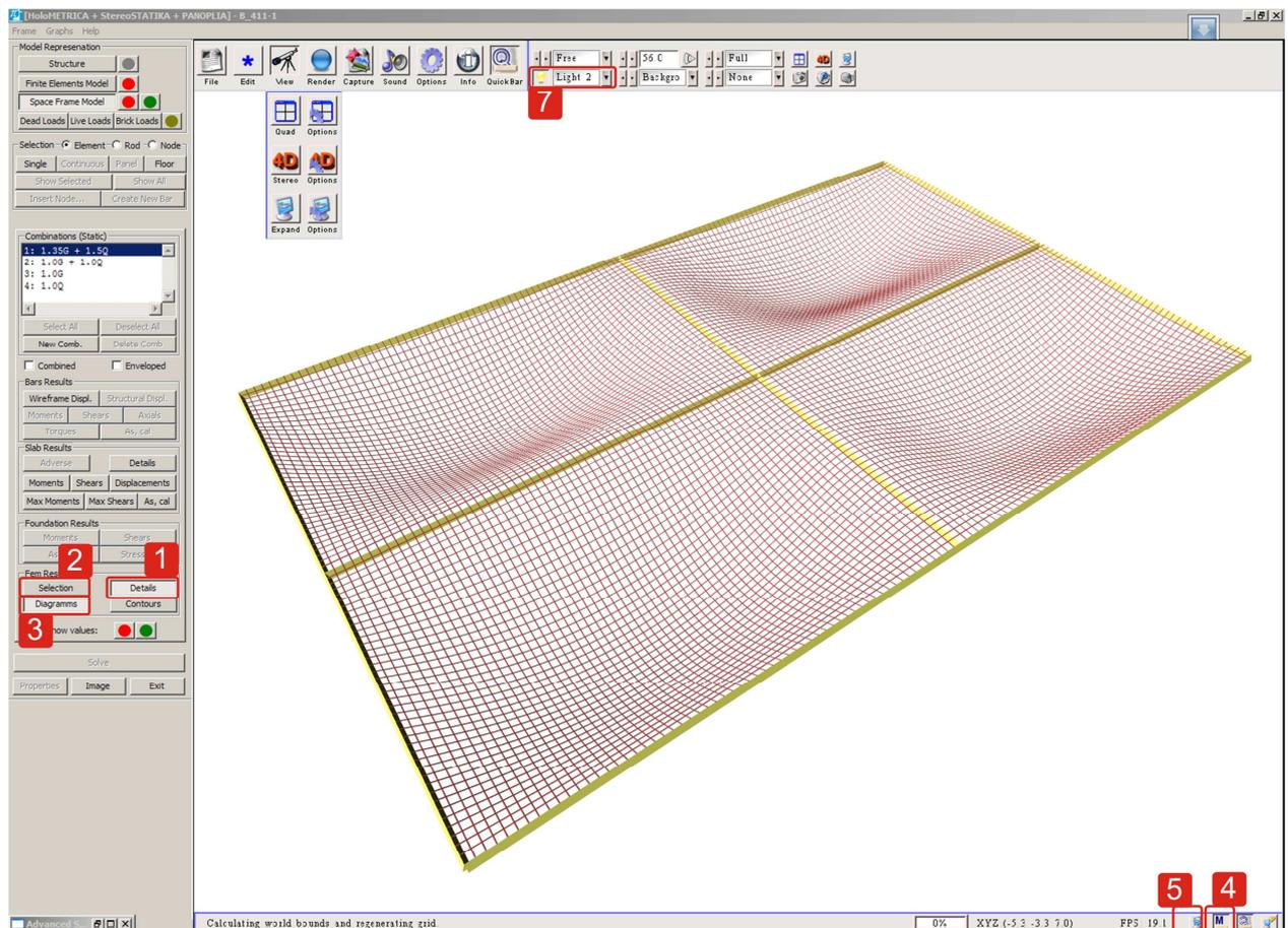
Figure 4.2.1-8: The following button sequence displays the 3D deformation of the structure:
