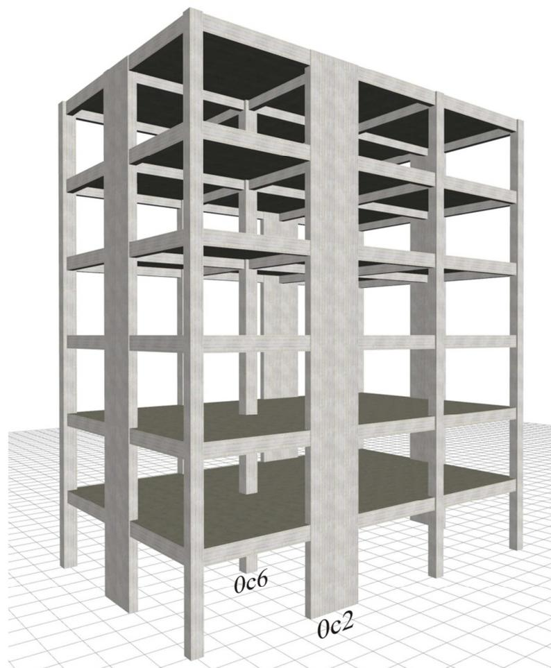
Figure 6.4.2-1: Structure comprising only columns and perimeter walls, project <B\_642-1>
