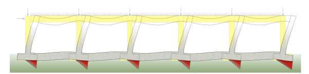
2. The earthquake causes reverse stresses in every part of a connecting beam thus applying almost the same flexure at the upper and the lower fiber.
