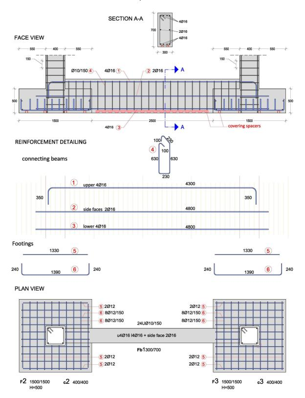
Foundation reinforcement of a two-column frame cproject: foundation121>
